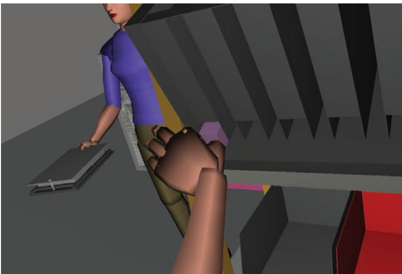
Jack human simulation model holding the part. Inset shows view from operator eyes.
