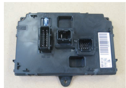
Modules of the Peugeot 407 project. Rear electronic control unit is placed under the bodywork in the rear of the car.
