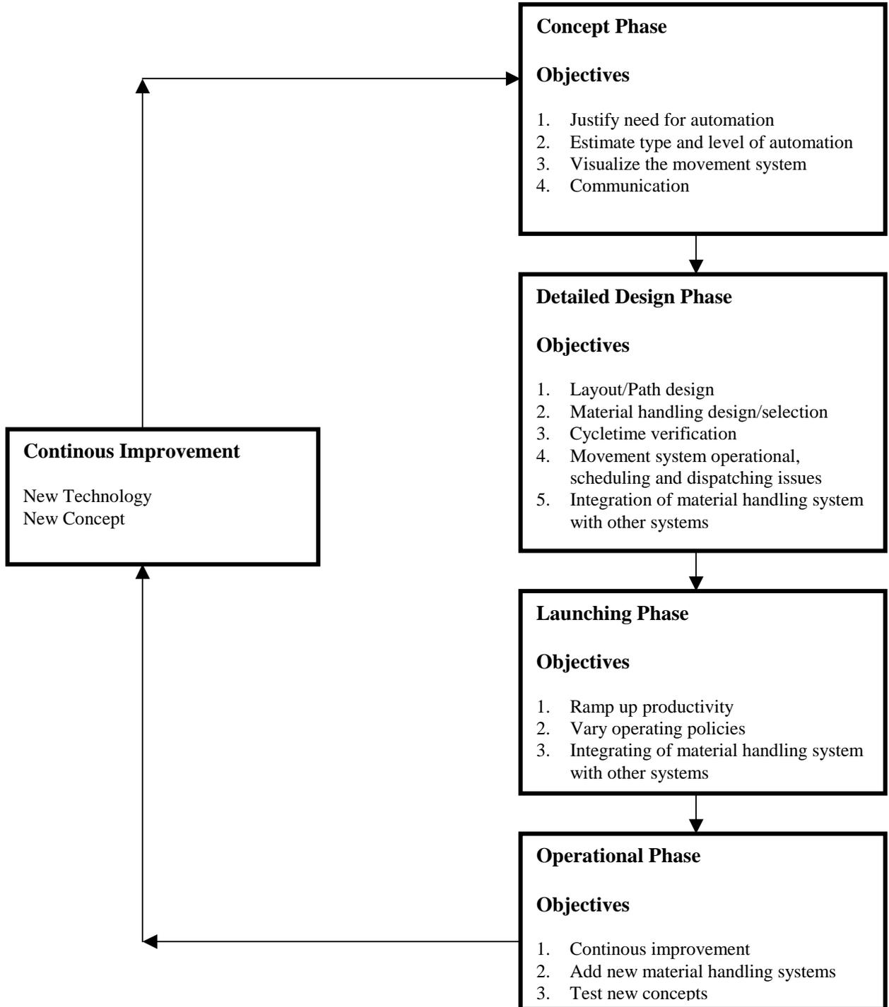
Figure 1: Application of Simulation to the four phases of a Material Handling project
