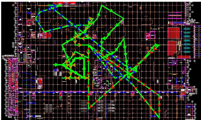
Figure 1: Activity "plotted" on plant layout to show the "spatial extent of activities" - used as a possible guideline to "combine responsibilities".
